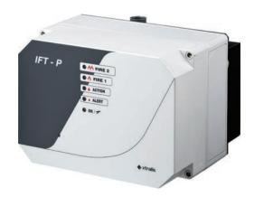
The ICAM IFT-P detector is an air-sampling system with an alarm sensitivity range from 0.01% to 20% obscuration/m (0.003% to 6.10% obscuration/ft). This detector is classified as a Very Early Warning Smoke Detector that can reliably detect fire at an early stage, and low to high concentrations of smoke over an area of up to 2000  $\text{m}^2$  (21 500  $\text{ft}^2$ ).
