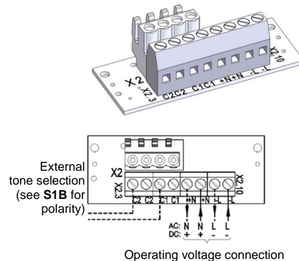
Common connection of flashing light and sounder
