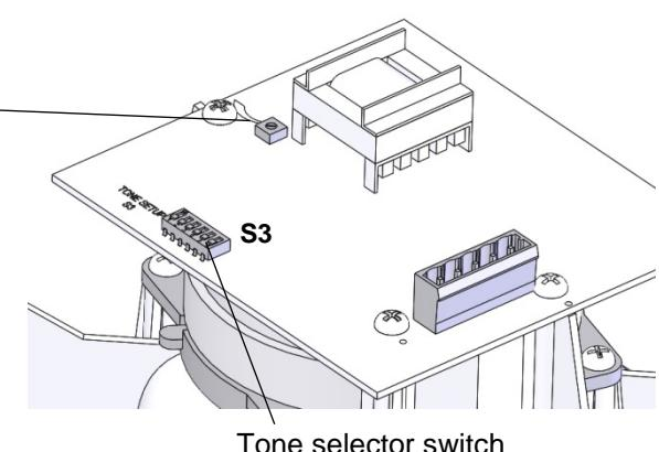
The desired tone can be selected using the **S3** tone selector switch. The tone is generated after the supply voltage is applied. A complete tone type table can be found in the Annex. See the digital operating instructions for the external control of other tones, source: [www.pfannenberg.com/manuals](http://www.pfannenberg.com/manuals).
